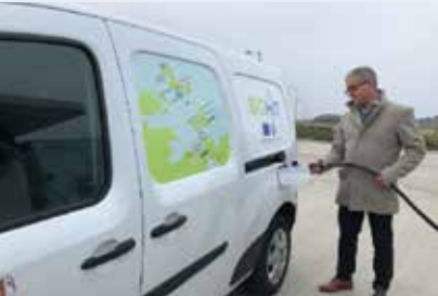
The Renault Kangoo BEV van, pictured here operating on the Orkney Islands has been converted to a range extended battery/FCEV.
