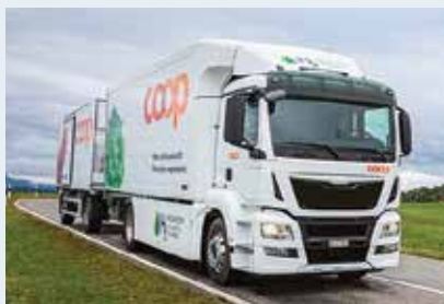
Esoro and Coop has developed a 34 Ton refrigerated demonstration truck with a 400km range.
