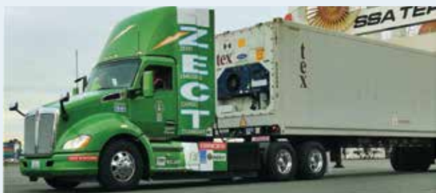
Kenworth & Ballard are testing a fuel cell drayage truck in Port of LA
