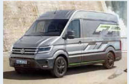
Volkswagen Crafter HyMotion concept carries 7.5 kg hydrogen tanks to cover ranges exceeding 500 km. Fuel consumption is 1.4 kg/100 km and re-fuelling takes four minutes. It will carry the same payload as it's diesel equivalent (up to 3T). It is based on the same electric drive train as eCrafter battery electric van but significantly improves on the eCrafter's max range of 160 km and max payload of 1.7T.
