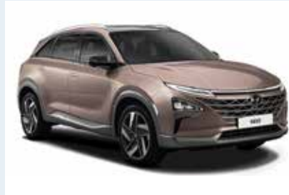
Hyundai Nexo will be available in Australasian markets in early 2019. It has 6.3kg hydrogen storage and a range of 600-800km on a 3-5 minute refill.
